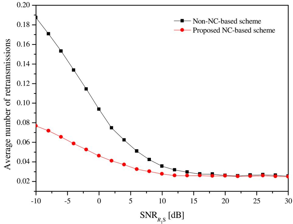
Fig. 5. Average number of data retransmissions per packet versus  $SNR_{R1S}$  for Scenario 1.
