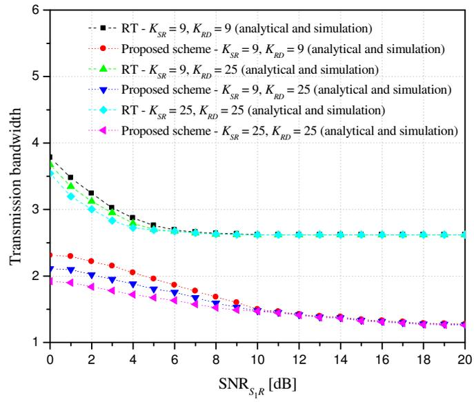
Figure 6: Transmission bandwidth of different protocols over Rician fading channels  $\mathcal{S}_i \rightarrow \mathcal{R}$  and Rician fading channels  $\mathcal{R} \rightarrow \mathcal{D}_i$  ( $i = 1, 2$ ) with various  $\mathcal{K}$  factors as a function of  $\text{SNR}_{S_1R}$ .
