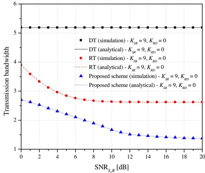
Figure 4: Transmission bandwidth of different protocols over Rician fading channels  $\mathcal{S}_i \rightarrow \mathcal{R}$  and Rayleigh fading channels  $\mathcal{R} \rightarrow \mathcal{D}_i$  ( $i = 1, 2$ ) as a function of  $\text{SNR}_{\mathcal{S}_1\mathcal{R}}$ .
