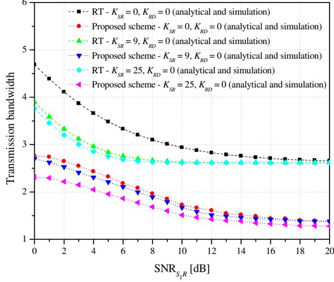
Figure 5: Transmission bandwidth of different protocols over Rician fading channels  $\mathcal{S}_i \rightarrow \mathcal{R}$  and Rayleigh fading channels  $\mathcal{R} \rightarrow \mathcal{D}_i$  ( $i = 1, 2$ ) with various  $\mathcal{K}$  factors as a function of  $\text{SNR}_{\mathcal{S}_1\mathcal{R}}$ .
