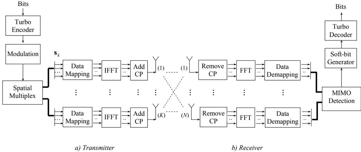
Fig. 1. Block diagram of a MIMO-OFDMA LTE downlink.
