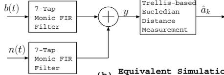
(b) Equivalent Simulation Model with Minimum Euclidian Distance Measurement
