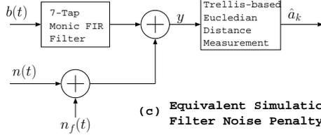
(c) Equivalent Simulation Model with Filter Noise Penalty
