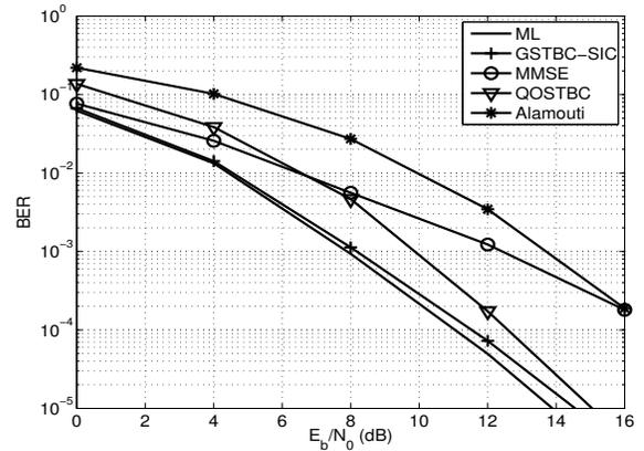
Fig. 2. BER performance comparison with different schemes.
