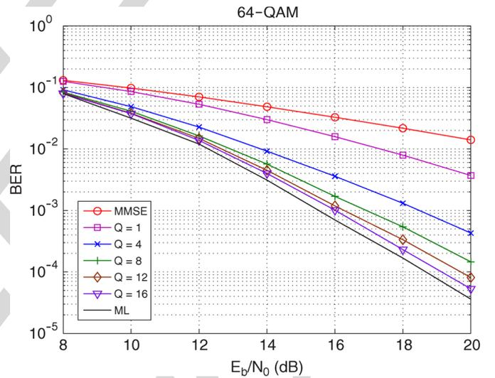
Fig. 4. BER performance of a  $4 \times 4$  MIMO system with 64-QAM signaling.
