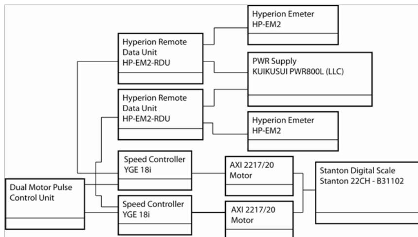
Fig. 10. Block diagram of co-axial the test-rig.
