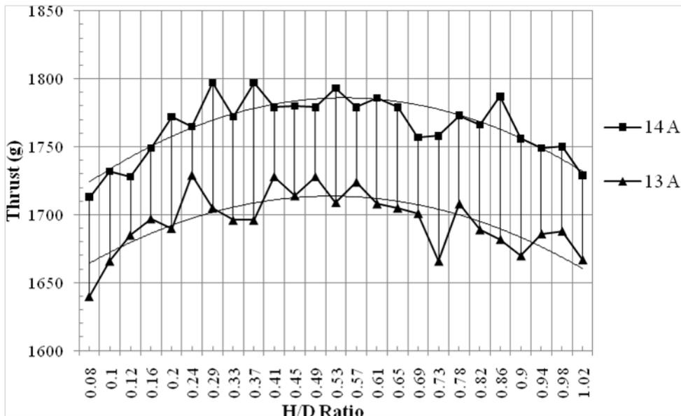
Fig. 13. Variation of co-axial thrust with rotor spacing.
