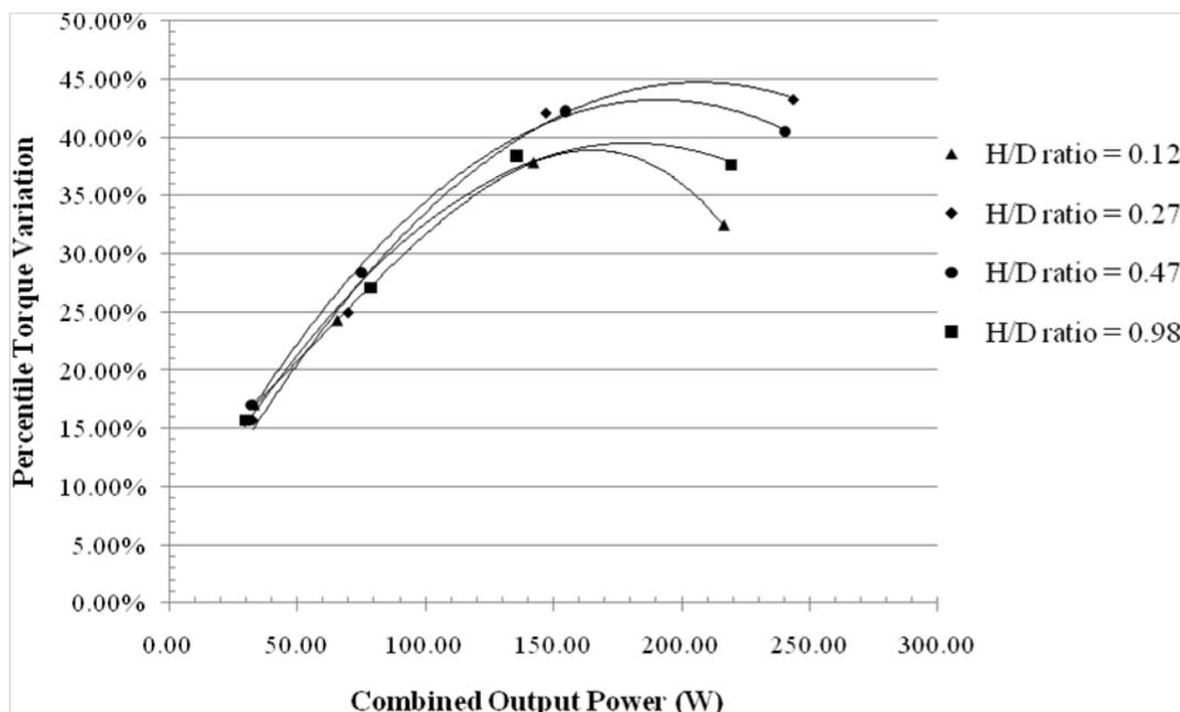
Fig. 15. Percentile torque variation versus combined output power.
