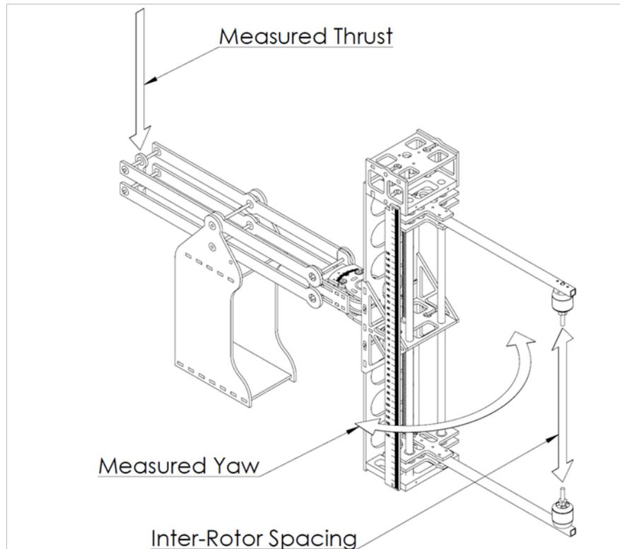
Fig. 8. CAD Model of the Co-Axial Test-Rig [23].
