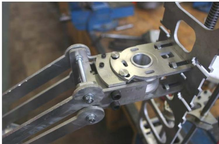
Fig. 9. Yaw mechanism attached to thrust bracket.
