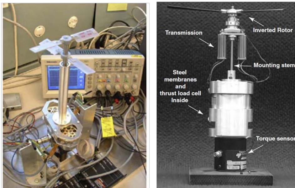
Fig. 7. muFLY [3] & UMD MICOR co-axial rotor system test-rigs [31].
