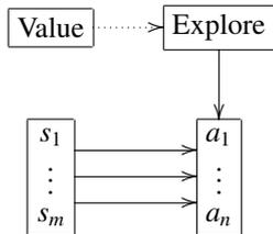
Figure 1: Components and connections of the Value and Explore modules controlling Hebbian learning of connections between CAs in modules  $S$  and  $A$ . Solid and dashed arrows show excitatory and inhibitory connections respectively.
