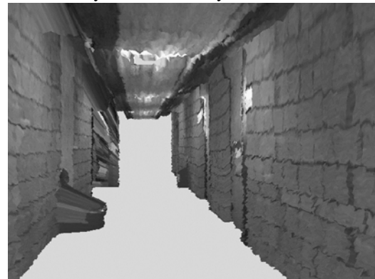
Figure 7: A corridor mapped using the Probabilistic On-Line Mapping system [12].
