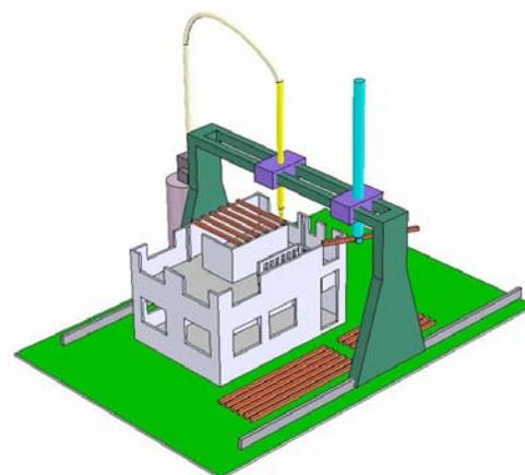
Figure 8: Construction of conventional buildings using CC [13].
