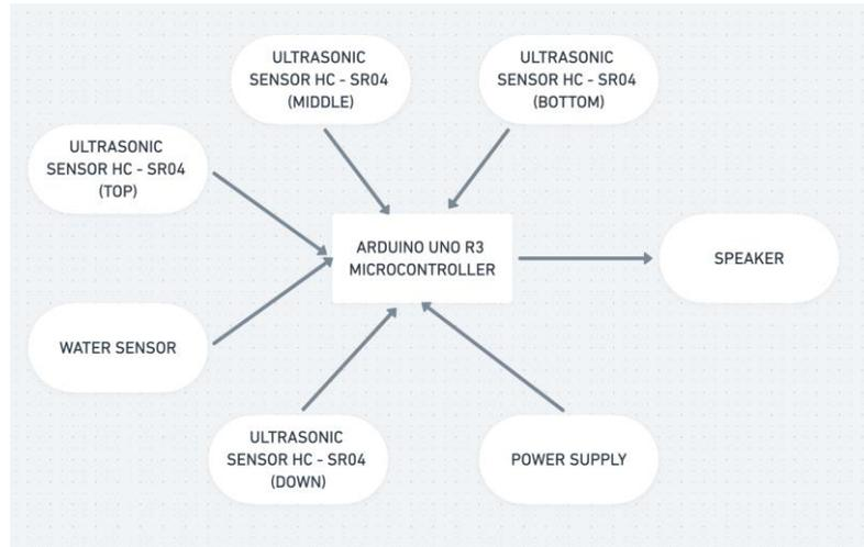
**Fig1:** Block diagram of the sub-system for obstacle detection
