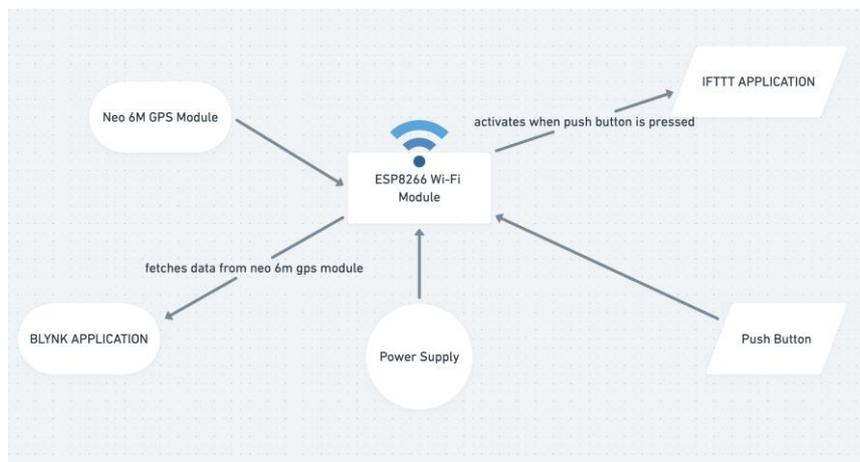
**Fig2:** Block diagram of the sub-system for location tracking
