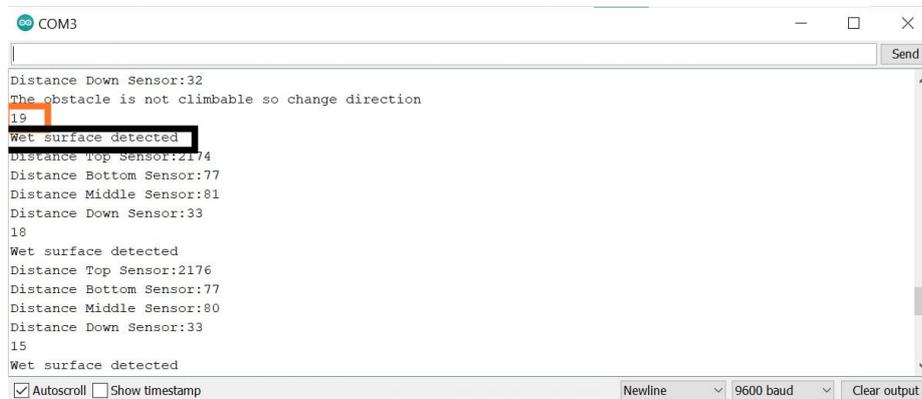
**Fig4:** Wet Surface Detection
