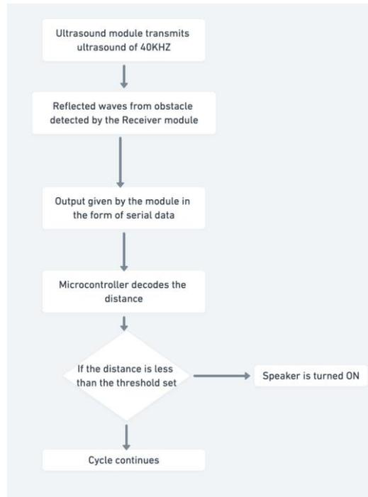
**Fig3:** Interaction of each Ultrasonic Sensor
