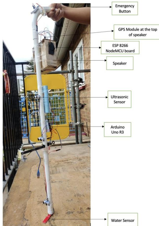
**Fig3:** Complete IoT-based Smart Navigation-Aid for Visually Impaired
