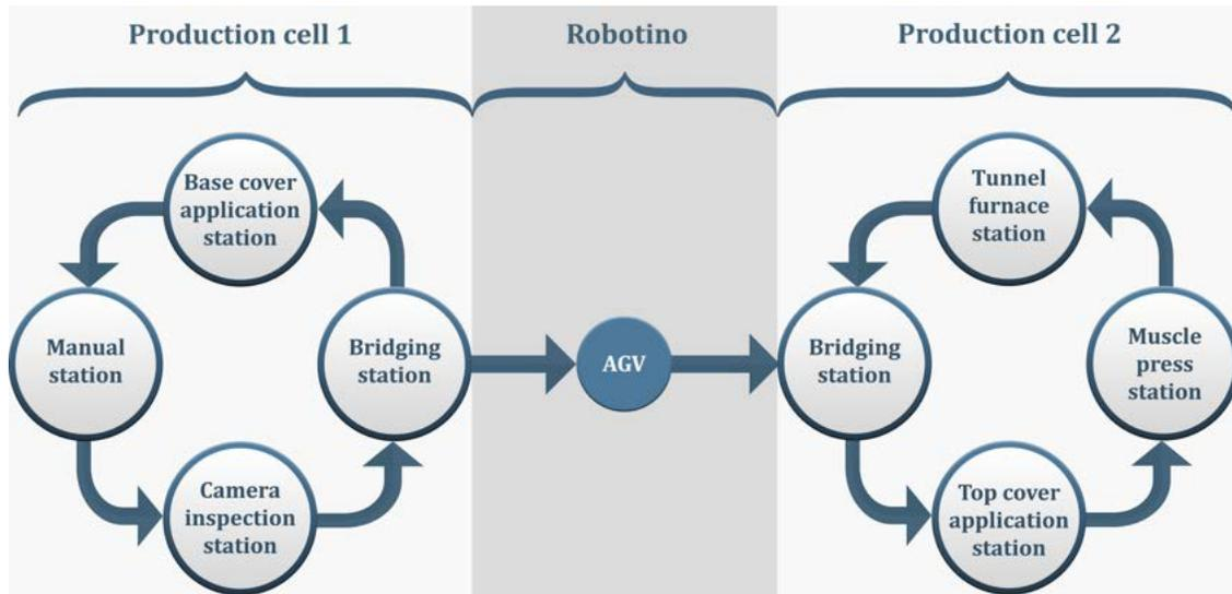
Fig. 1: Festo Cyber Physical Factory functional diagram.
