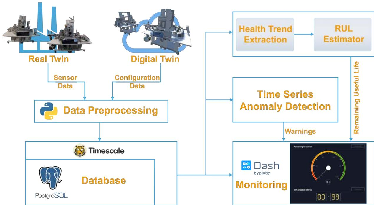
Fig. 4: A Digital Twin framework for Predictive Maintenance.
