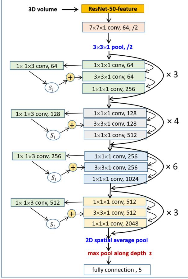
Figure 3. The depth-ResNet architecture applied in this paper, where  $\times N$  at each conv level refers to the block (e.g. conv5\_x) repeats  $N$  (e.g. 3) times consecutively.
