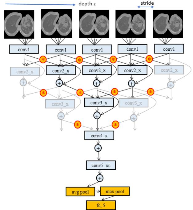
Figure 4. A block in the depth-ResNet that is applied in the paper.
