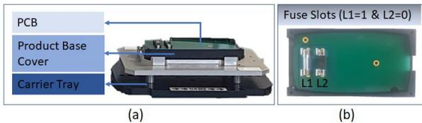
Figure 5. Product Base Carrier Tray (a) Product state after station 2 (b) Top view of PCB with fuse slots
