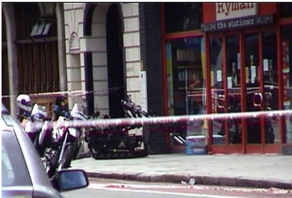
Fig. 2. Wheelbarrow Revolution inspecting a suspect package
