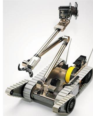
Fig. 3. The Packbot UGV developed by iRobot.
