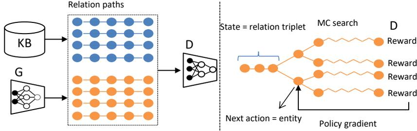
Figure 1: Proposed mh-RGAN architecture. **Left:**  $D$  is trained over the real and generated relation paths. **Right:**  $G$  is trained via policy gradient for which the final reward signal is provided by  $D$  and is passed back to the intermediate action value via Monte Carlo search.
