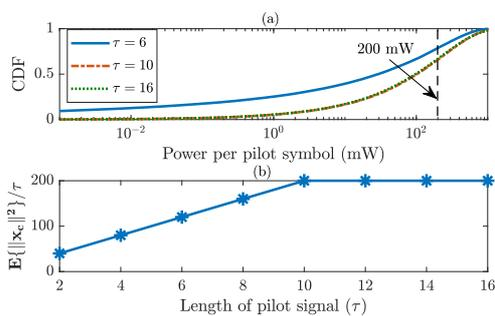
Figure 2. (a) The CDFs of the power allocated for each pilot symbol of the proposed approach with different pilot lengths; (b) The average power allocated for each pilot symbol of the proposed approach v.s. the pilot length.
