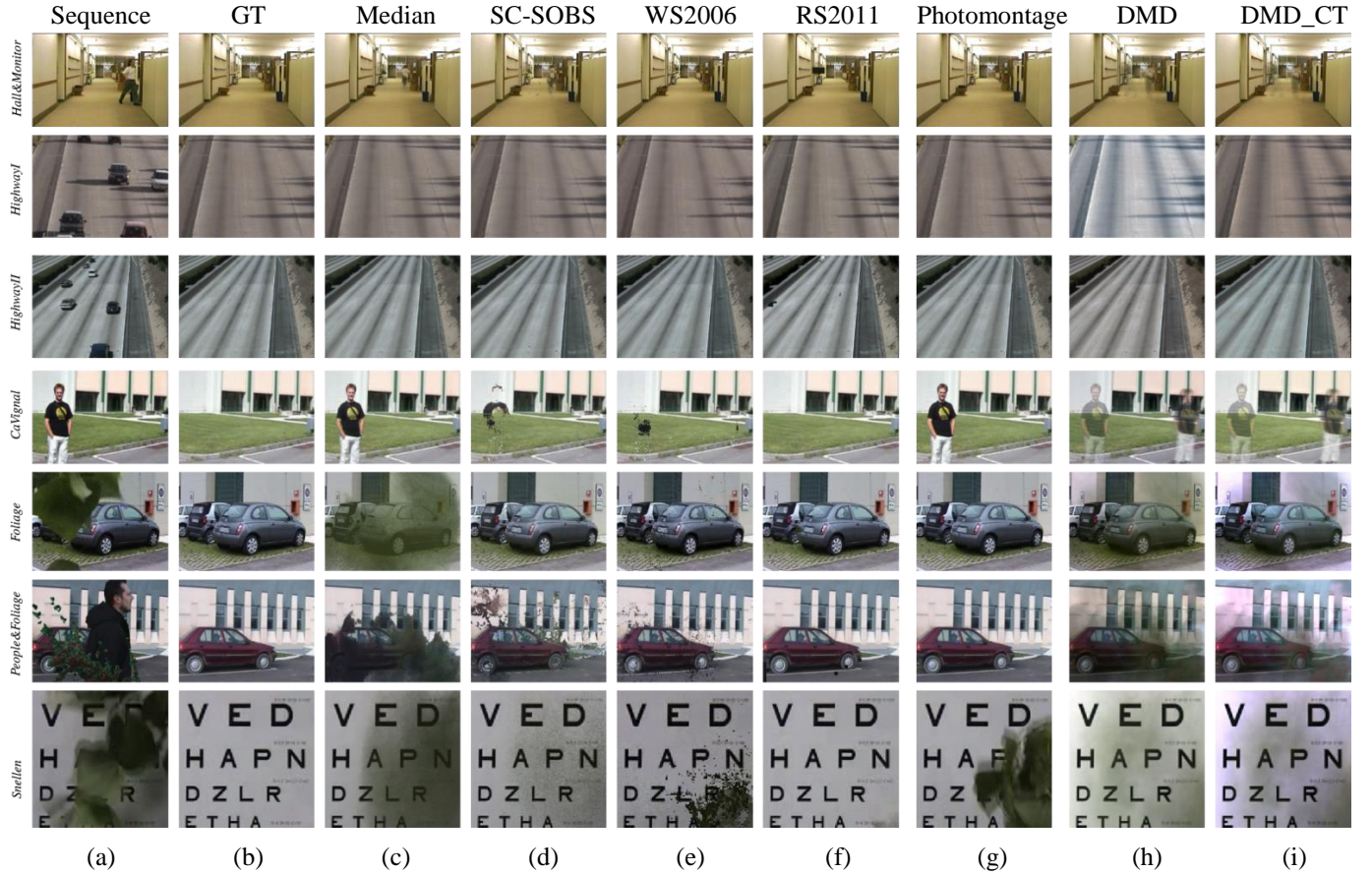
Fig. 2. (a) Exemplar frames corresponding to {295, 0, 0, 0, 261, 10, and 0} from seven different sequences of the SBI dataset. (b) Corresponding GT’s for the sequences. (c-g) Background models generated by benchmarked methods: (c) Median, (d) SC-SOBS, (e) WS2006, (f) RS2011, (g) Photomontage. (h) DMD and (i) DMD_CT. Both DMD and DMD_CT are the proposed methods in this paper. The images {a-g} are taken from [1].
