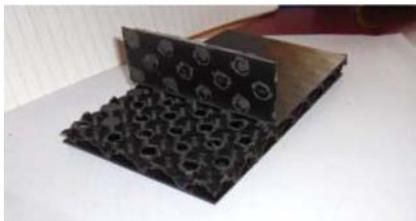
Fig. 14. Polypropylene thermal absorber with honeycomb structure for PV/T module [31].
