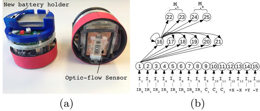
**Fig. 1.** (a) The e-puck robot with optic-flow sensor. (b) The robot's controller. The continuous line arrows indicate the efferent connections for only one neuron of each layer. Hidden neurons receive an afferent connection from each input neuron and from each hidden neuron, including a self-connection. Output neurons receive an afferent connection from each hidden neuron. Sensors to sensor neurons correspondence is indicated underneath the input layer.
