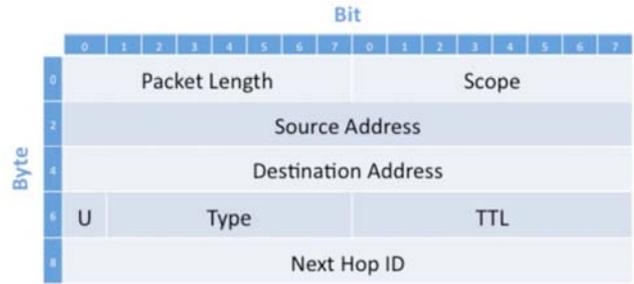
Figure 8. SDN-WISE Packet Header [26].
