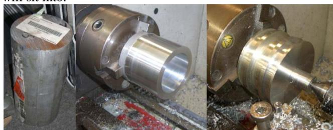
Fig. 7 Turning down process.
