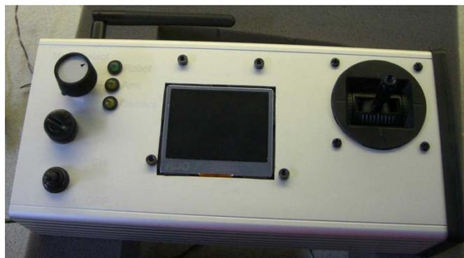
Fig. 6 Ground Control Unit with joystick for arm articulation and system locomotion.
