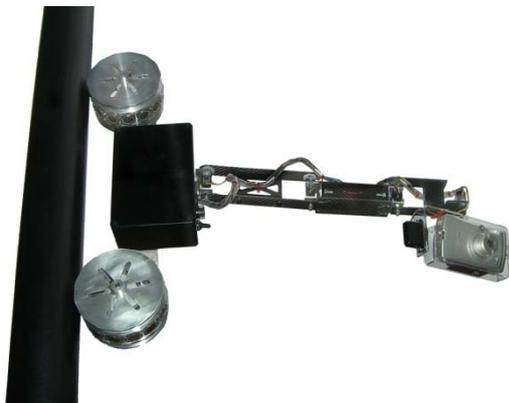
Fig. 5 PC-101 attached to lighting column.
