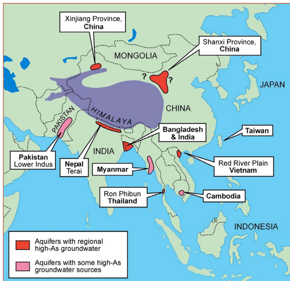
Figure 5: Arsenic contamination in Asia [question marks indicate uncertain concentrations in Shanxi Province, China] BGS (Smedley, 2003).
