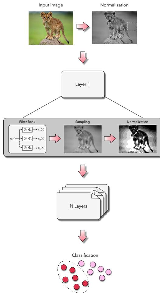
**Fig. 1** A typical Convolutional Neural Network architecture.
