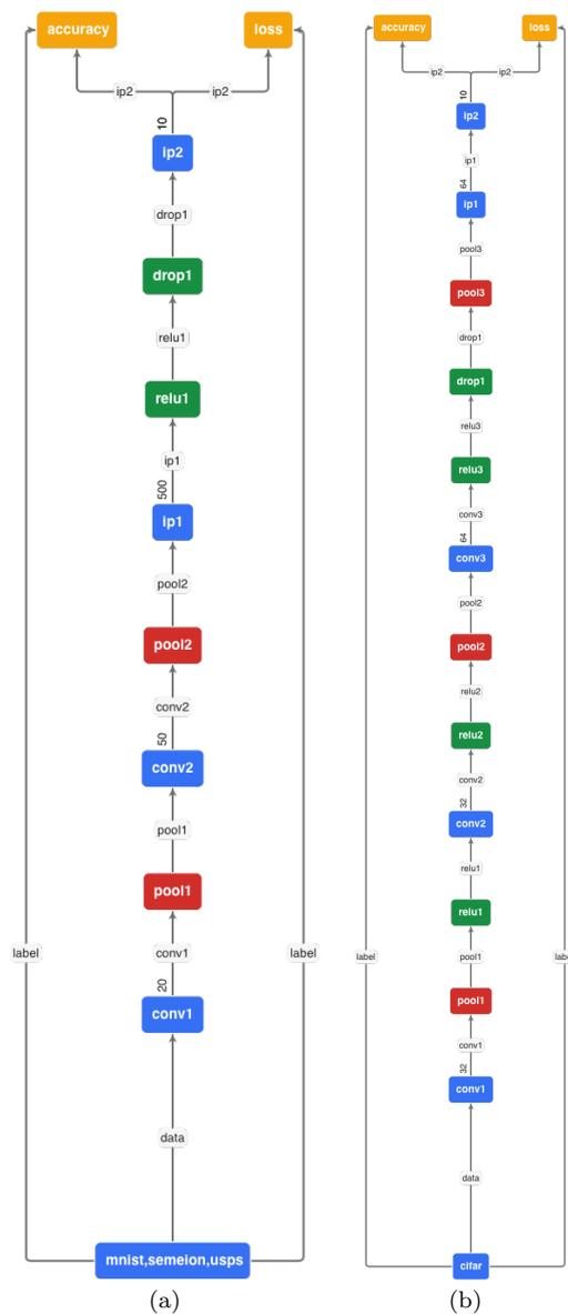
**Fig. 3** CNN architectures for: (a) MNIST, Semeion and USPS, and (b) CIFAR-10 datasets. The picture was generated with the following tool: [http://yanglei.me/gen\\_proto/](http://yanglei.me/gen_proto/).
