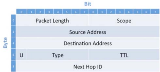
Figure 8. SDN-WISE Packet Header [26].
