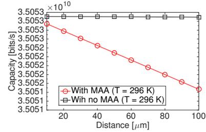
Fig. 5. Channel capacity versus distance between two antennas.
