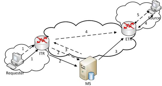
Figure 4. Proxy-Enabled (solid arrows).No Proxy-Enabled (dashed arrows)
