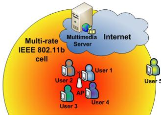
Figure 4. Simulated network topology for scenario 1
